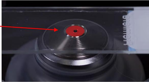
15. Set the microscope with one fluorescent setting (i.e. **Fluo** → **DAPI**, etc.) on touchscreen → turn Z dial (still on precise and fine movements) **counterclockwise** to lower the lens → keep lowering lens until you find sample through eyepieces on microscope
