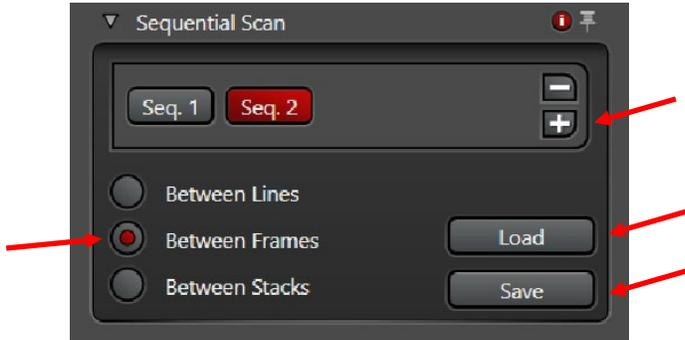
22. **STOP** live imaging → go to **Seq. 2** and **turn off** everything: turn **OFF** the detector → decrease the laser intensity to **0%** → **CLOSE** shutter → **DESELECT** that laser
